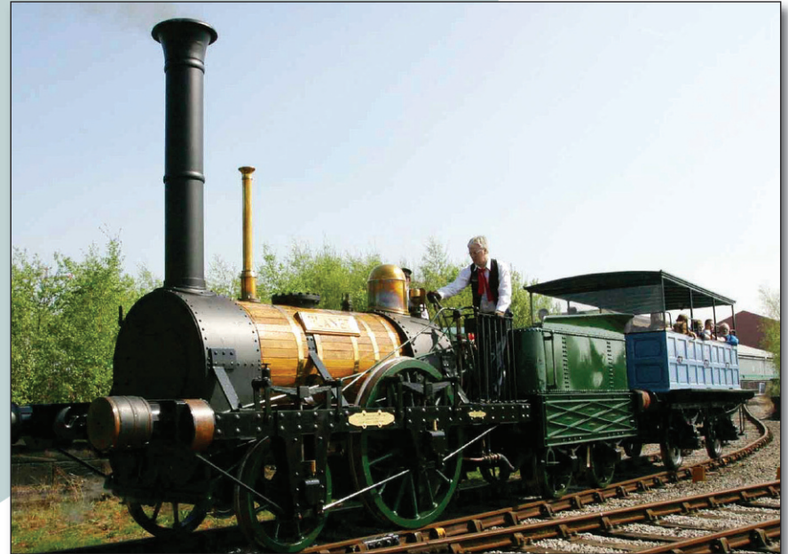
Planet , a 2-2-0 built by Robert Stephenson in 1830 for the Liverpool & Manchester Railway, was the first locomotive to employ inside cylinders. A working replica was built by the Friends of the Museum of Science and Industry in Manchester in 1992.
