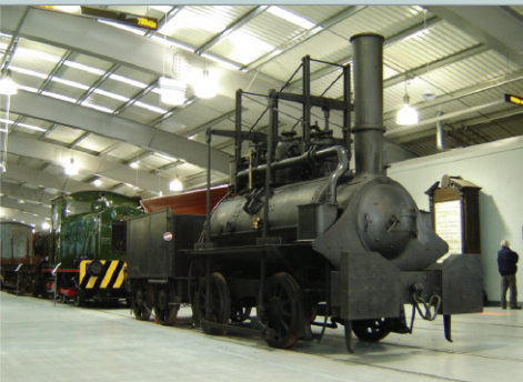
Planet , a 2-2-0 built by Robert Stephenson in 1830 for the Liverpool & Manchester Railway, was the first locomotive to employ inside cylinders. A working replica was built by the Friends of the Museum of Science and Industry in Manchester in 1992.
